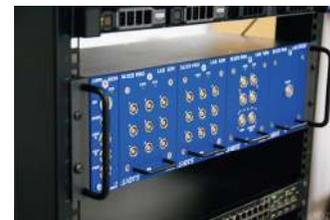
SLICE PRO LAB fits into a standard 19 inch rack configuration.
