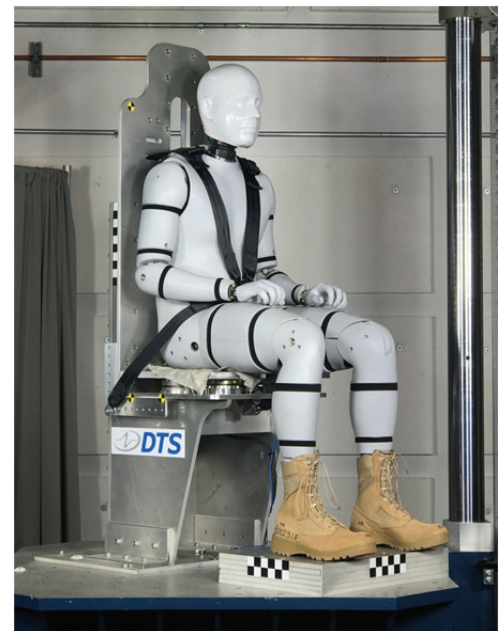
WIAMan with 146 SLICE6 HB channels
