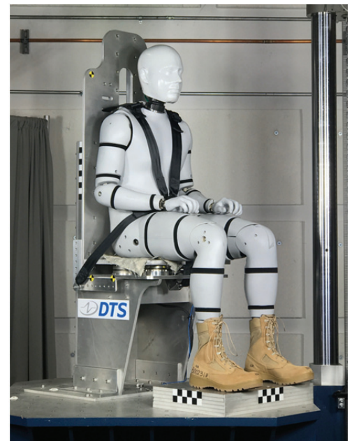
WIAMan with 146 SLICE6 HB channels
